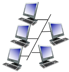
shared wire (e.g., cabled Ethernet)
